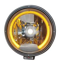
For many years, the SIM halogen long beam light has been a fixed value on many trucks throughout Europe. In order to meet your demand for a long beam light with amber position light this new version with LED was developed.
